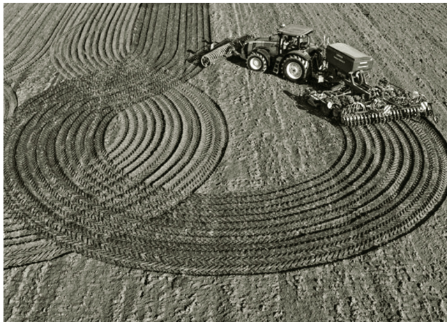
FIGURE 5.13 John Deere’s iTEC Pro for hands-free turns and implement control at headlands. (Photo courtesy of Deere & Company.)
