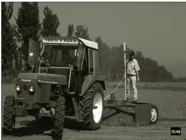
FIGURE 8.31 Land leveler in operation.
