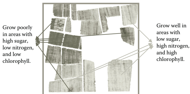
FIGURE 3.10 (See color insert.) Pseudocolor composition map of biochemical parameters, including chlorophyll, total nitrogen, and soluble sugar. Red lines: The crops grow poorly in areas with high sugar, low nitrogen, and low chlorophyll. Green lines: The crops grow well in the areas with low sugar, high nitrogen, and high chlorophyll. (From Liu, L.Y. 2002. Hyperspectral Remote Sensing Application in Precision Agriculture . Postdoctoral research report of Institute of Remote Sensing Applications, Chinese Academy of Sciences. With permission.)
